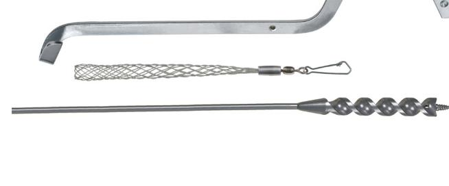
Klein's Flex Bit kit includes everything you need for drilling and pulling wire and cable in-wall. The flexible drill bit makes 9/16-Inch (14 mm) holes in wood. The folding placement tool helps guide the bit as you drill. The pulling grip attaches to the flexible drill bit after the hole has been made to pull wire and cable through.
