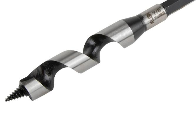
The deep, open-throat design of the Ship Auger bit clears chips for faster, cleaner cuts. The shank is 7/16-Inch hex to fit 1/2-Inch (13 mm) and larger three-jaw chucks. Used for heavy construction and repair work in mines, on docks and bridges as well as electrical work.
