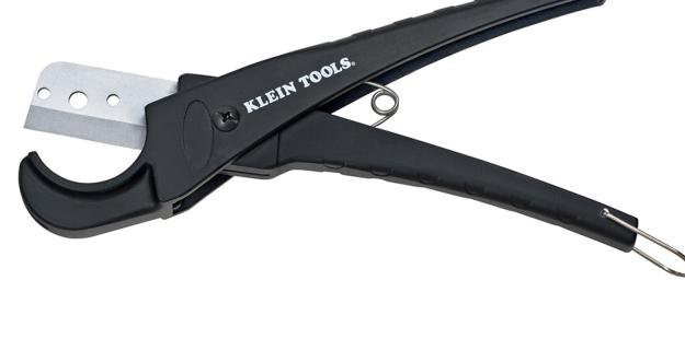
The Klein Tools 3/4 in. PVC Cutters are ideal for cleanly cutting schedule 40 PVC piping. They are crafted with steel for strength and feature 4 in. handles and a reversible blade for a longer cutting life. The cutters work well for cutting schedule 40 PVC piping with diameters up to 3/4 in. and flexible piping with diameters up to 1-3/8 in.
