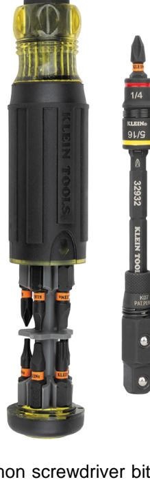
The 16-in-1 Impact Hybrid Screwdriver features the most common screwdriver bits and nut drivers in one tool. Use as a screwdriver or as an impact driver attachment. Multi-purpose flip socket on end of blade has three positions for multiple functions.
