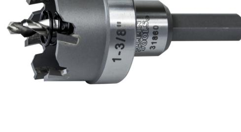
This carbide hole cutter cuts quick, precise holes in a variety of materials. Integrated flange prevents the operator from drilling beyond the sheet metal. Split point pilot drill bit prevents bit walking.
