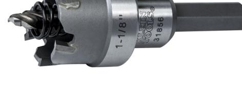
This carbide hole cutter cuts quick, precise holes in a variety of materials. Integrated flange prevents the operator from drilling beyond the sheet metal. Split point pilot drill bit prevents bit walking.
