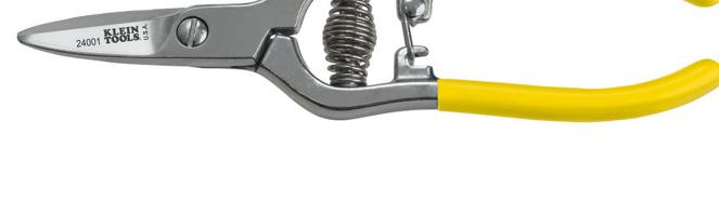
This Rapid-Cutting Snip is excellent for cutting stranded wire, light metal, cordage and Kevlar® insulation wire in fiber-optic applications. The spring-loaded design gives this snip self-opening action so less effort is required. It features one serrated blade for non-slip cutting action.
