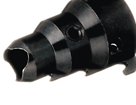
From Klein Tools, the Conduit Reamer works with a screwdriver to ream and smooth thin-wall conduit. It locks onto a screwdriver and can ream both ID and OD at the same time. Comes with two set-screws to fit either round or square-shank screwdrivers.
