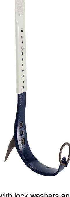
Secure sleeve and leg iron connection. 2 slotted hex-head bolts with lock washers and barrel-type nuts join the steel sleeve and leg iron together. Steel split ring secures ankle strap in place and allows for quick replacement.
