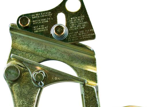
This parallel jaw grip was specifically designed to securely pull slippery HDPE-coated cable or tree wire. The innovative high-traction surface grips the cable without damaging the outer jacket. The tough carbide grit technology withstands even the harshest jobsite conditions. The grip is spring-loaded for one-handed operation and easy placement on the conductor.
