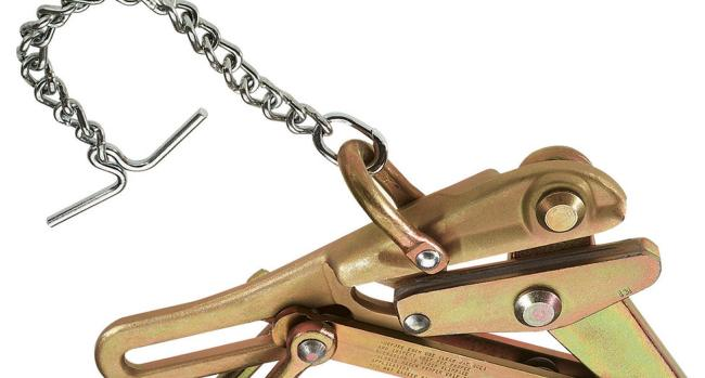
Designed for use on aluminum, copper, weatherproof coated wire, PVC covered conductors and messenger and guy strand. The Chicago style grip was designed for cable sizes from 0.12-Inch to 1.0-Inch (3.10 to 25.4 mm). Equipped with chain, toggle and shackle. For support wire 0.134-Inch and larger, refer to 1659 series. Outside diameter of support wire includes thickness of polyethylene coating.
