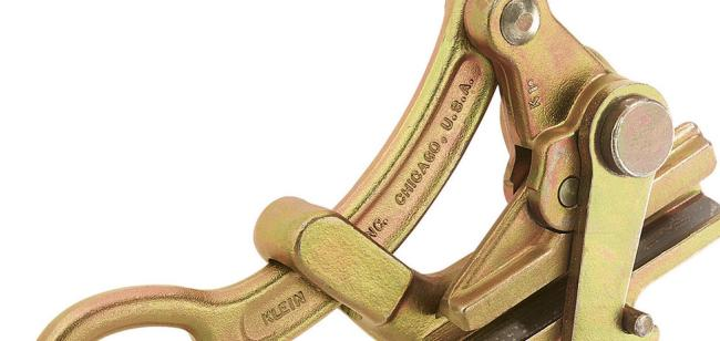
Longer jaws achieve a firm hold, reducing possibility of slippage and damage to cable. Design includes a latch, plus a large-diameter eye that accommodates large hooks on hoists, winches and tackle blocks. When latch is closed, it helps maintain cable position in grip jaws.
