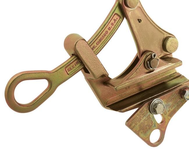
Lightweight, compact grips pull an exceptionally wide range of cable sizes and types. Designed with a round inside-jaw contour for maximum contact to minimize conductor damage. Lower jaw is serrated to firmly grip insulated cables and conductors. Design includes a latch that prevents the grip from falling in case of jaw disengagement from the cable.
