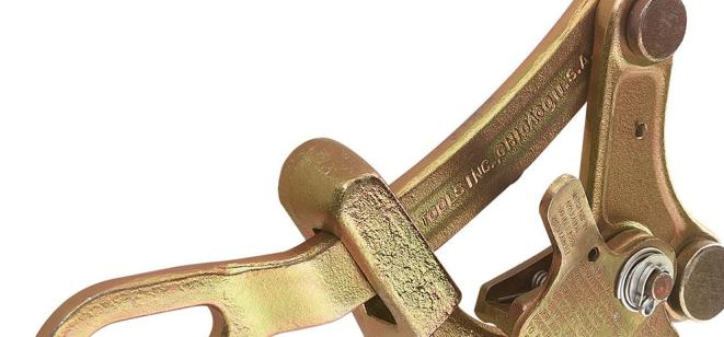
Lightweight, compact grips pull an exceptionally wide range of cable sizes and types. Designed with a round inside-jaw contour for maximum contact to minimize conductor damage. Lower jaw is serrated to firmly grip insulated cables and conductors. Design includes a latch that prevents the grip from falling in case of jaw disengagement from the cable.
