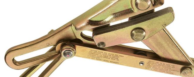
Designed for use on aluminum, copper, weatherproof coated wire, PVC covered conductors and messenger and guy strand. The Chicago style grip was designed for cable sizes from 0.12-Inch to 1.0-Inch (3.10 to 25.4 mm). When pulling EHS (extra-high-strength) galvanized-steel cable, the galvanizing has a tendency to coat the jaws of any grip, causing the cable to slip. Double V contour reduces the possibility of slippage and damage to the cable.
