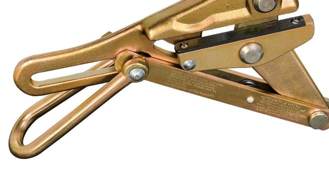
Designed for use on aluminum, copper, weatherproof coated wire, PVC covered conductors and messenger and guy strand. The Chicago style grip was designed for cable sizes from 0.16-Inch to 0.55-Inch (4.06 - 13.97 mm). Double V grooves give four-point contact, reducing chance of slipping and providing proper alignment of wire and cable.
