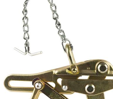
This Chicago Grip is designed specifically to work with coated guy strand and EHS cable. Klein grips are made of drop-forged, quality US steel and heat treated for strength and durability. The chain, toggle and shackle keep the grip from falling off the cable. The 5-Inch jaw length increases the surface area contact with the cable minimizing cable damage. The sawtooth jaw profile resists galvanization build-up.
