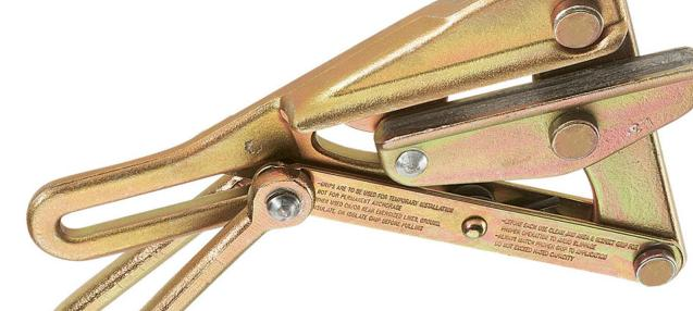
Designed for use on aluminum, copper, weatherproof coated wire, PVC covered conductors and messenger and guy strand. The Chicago style grip was designed for cable sizes from 0.218-Inch to 0.55-Inch (5.5 to 13.9 mm). Double V grooves give four-point contact, reducing chance of slipping and providing proper alignment of wire and cable.
