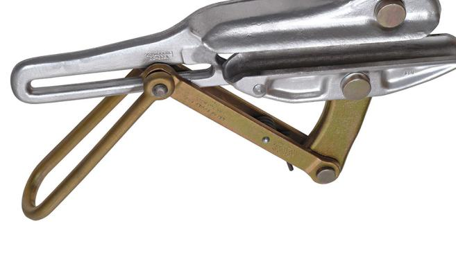
Klein Tools' 1628 Series Chicago Grips have a round inside jaw contour designed to hold weatherproof strand and solid coated wire. They also have a notched jaw to provide a firm grip on insulation. All Klein grips are manufactured from custom drop-forged steel that is machined and heat treated for excellent durability. Each grip is individually hand inspected and actuated for proper function. Grips are also rigorously tested and pulled to rated load to ensure the highest quality and reliability.
