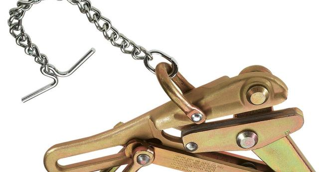
The Klein Tools 1628-16AT Chicago Grip is identical to a Bell-System type H Strand Puller. It is equipped with a chain, toggle and shackle to keep the grip from falling off the cable. All Klein grips are manufactured from custom drop-forged steel that is machined and heat treated for excellent durability. Each grip is individually hand inspected and actuated for proper function. Grips are also rigorously tested and pulled to rated load to ensure the highest quality and reliability.
