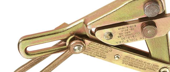
Klein Tools' 1613 Series Bare Wire Chicago Grips are designed to work with solid and stranded bare wire from 0.08-Inch to 0.20-Inch (2 mm to 5.1 mm). All Klein grips are manufactured from custom drop-forged steel that is machined and heat treated for excellent durability. Each grip is individually hand inspected and actuated for proper function. Grips are also rigorously tested and pulled to rated load to ensure the highest quality and reliability.
