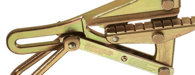
Klein Tools' 1611 Series Chicago Grips have a round inside jaw contour designed to hold weatherproof strand and solid coated wire. They also have a notched jaw to provide a firm grip on insulation. All Klein grips are manufactured from custom drop-forged steel that is machined and heat treated for excellent durability. Each grip is individually hand inspected and actuated for proper function. Grips are also rigorously tested and pulled to rated load to ensure the highest quality and reliability.
