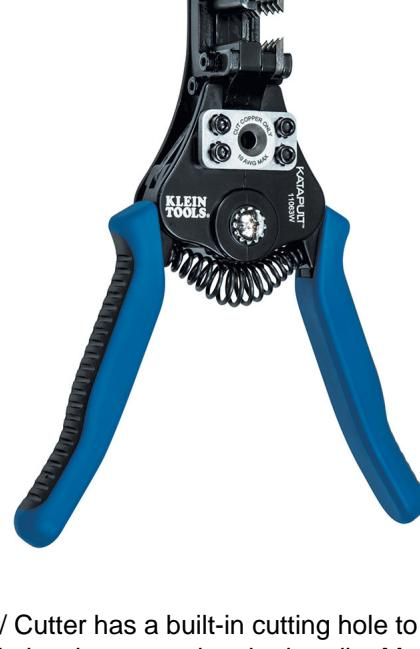
Klein Tools' Katapult® Solid and Stranded Wire Stripper / Cutter has a built-in cutting hole to cleanly cut 8-20 AWG solid and 10-22 AWG stranded wire, while the stripping head allows you to easily grip and strip just by squeezing the handle. Made of cast alloy with a heavy-duty Ecoat finish for corrosion resistance and durability.
