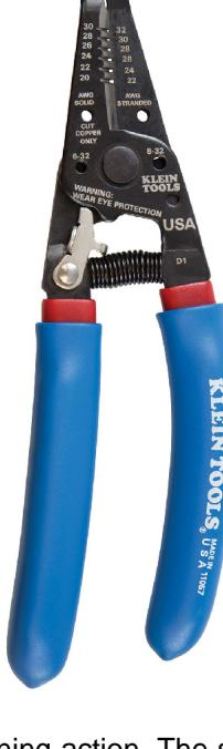
Klein's Wire Stripper/Cutter features a coil spring for fast self-opening action. The strong-gripping serrated nose allows for easy bending, shaping and pulling of wire. The Wire Stripper/Cutter has precision-ground stripping holes and screw-shearing holes. For use with 20-30 AWG Solid and 22-32 Stranded wire.
