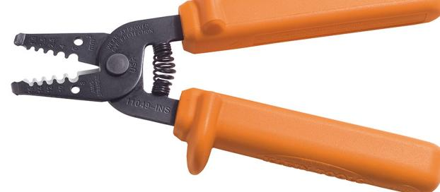
This compact, lightweight wire-stripping, cutting tool cuts, strips, loops and gauges solid wire. Dual layer orange-over-white insulation protects against electric shock. Meets or exceeds ASTM F1505-10, IEC 60900: 2004, CAN/ULC-60900-09, NFPA 70E, 2011 ed., CSA Z462 standards for insulated tools, and are clearly marked with the official 1000-volt rating symbol. Hardened spring steel with precision-ground stripping holes for easy removal of insulation.
