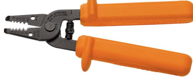
This compact, lightweight wire-stripping, cutting tool cuts, strips, loops and gauges 10-18 AWG solid wire. Dual layer orange-over-white insulation protects against electric shock. Exceeds IEC 60900 and ASTM F1505 standards for insulated tools, and are clearly marked with the official 1000-volt rating symbol. Hardened spring steel with precision-ground stripping holes for easy removal of insulation.
