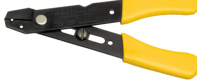
Klein Tools' 1003 Wire Stripper and Cutter is a handy, light, compact tool for stripping 12-26 AWG solid and 14-28 AWG stranded wire. Features convenient hole for looping or bending wire. Adjustable slide stop with set screw for repeat stripping work.
