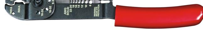
This Multi Tool performs 6 different functions with the same tool. It gauges, cuts and strips wire, measures and shears machine screws and crimps insulated terminals and connectors. Use the threaded holes to easily measure the size of a machine screw and cut it if needed. The plastic-covered handles are cushioned for added comfort.
