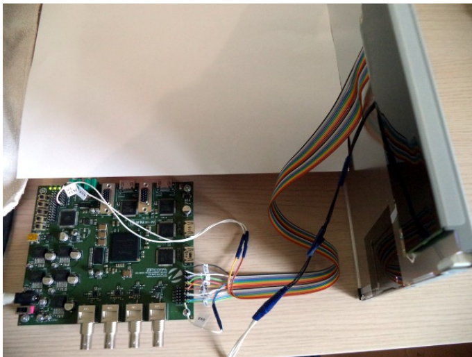
Figure 6: Demo setup with the Zipcores HD-Video board
