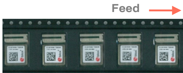
Figure 14: Orientation of NINA-W152/NINA-W156 module on tape
