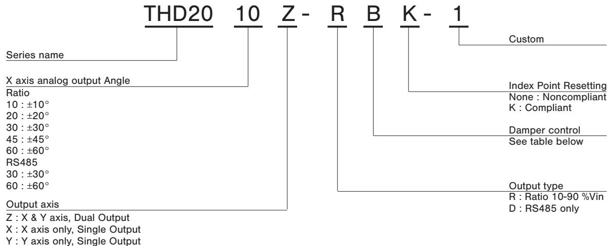
※ Cut-off frequency and Time constant against Damper time constant are shown the below table.
