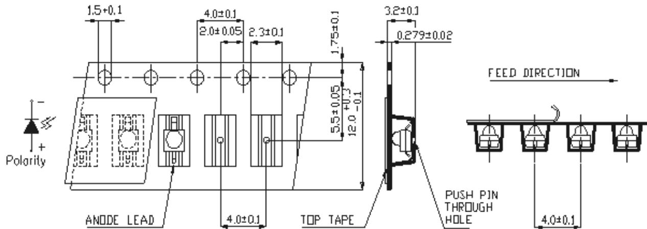
Note: The tolerances unless mentioned are  $\pm 0.1$ , unit=mm.
