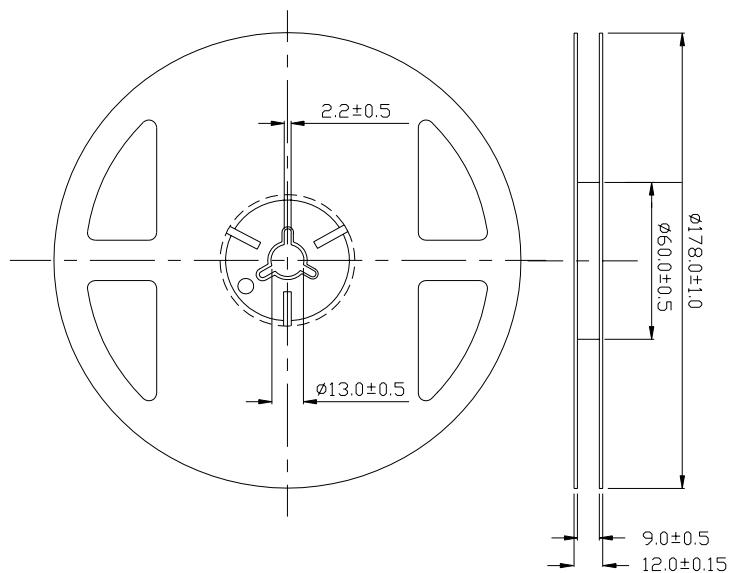
**Note:** The tolerances unless mentioned is  $\pm 0.1\text{mm}$  ,Unit = mm**19-237/R6GHBHC-A01/2T**
