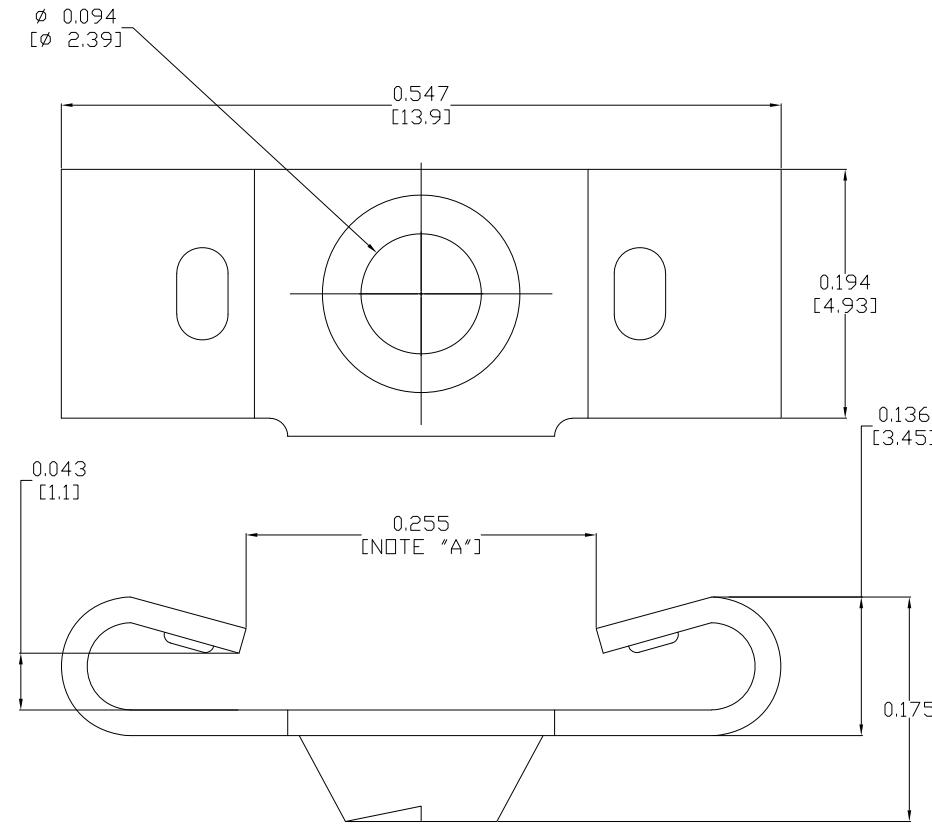
NOTE "A" - FLEXIBLE SPRING STEEL ALLOWS RETENTION FOR DIFFERENT CONNECTOR THICKNESS
