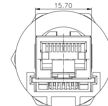
Nut - Torque Spec (0.56 Nm)
