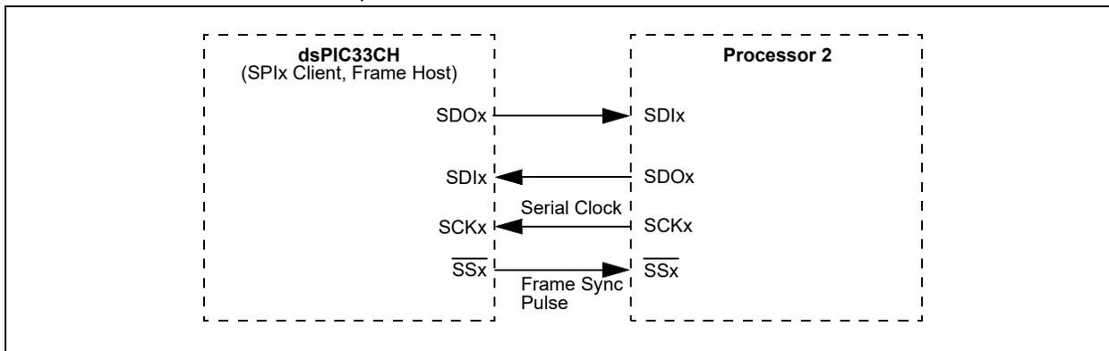
**FIGURE 14-8: SPIx CLIENT, FRAME CLIENT CONNECTION DIAGRAM**
