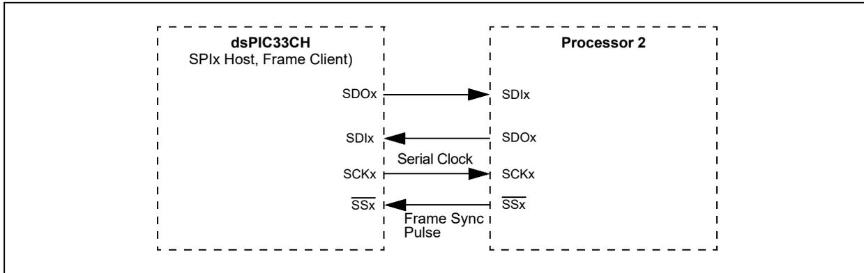
**FIGURE 14-7: SPIx CLIENT, FRAME HOST CONNECTION DIAGRAM**
