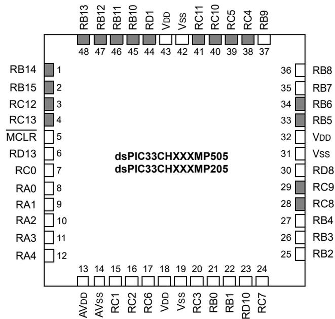
**Note 1:** Shaded pins are up to 5.5 Vdc tolerant (refer to [Table 3-29](#)). For the list of analog ports, refer to [Table 3-28](#) and [Table 4-25](#).
