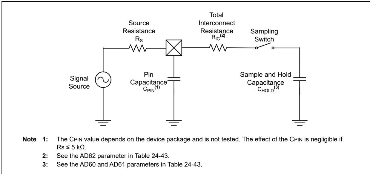
The total acquisition time for the Analog-to-Digital conversion is a function of the Holding Capacitor ( $C_{HOLD}$ ) charge time. For the ADC module to meet its specified accuracy, the Holding Capacitor ( $C_{HOLD}$ ) must be allowed to fully charge to the voltage level on the analog input pin. The Signal Source Impedance ( $R_s$ ) and the Interconnect Impedance ( $R_{IC}$ ) combine to affect the time required to charge the  $C_{HOLD}$ . The total
