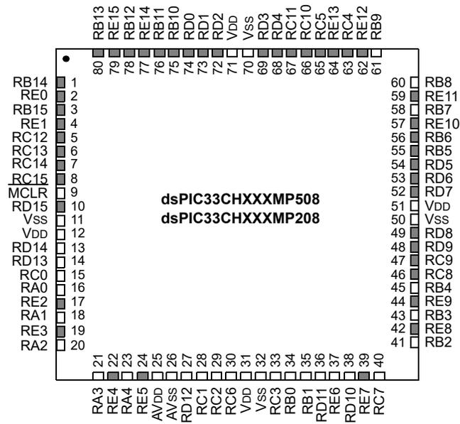
**Note 1:** Shaded pins are up to 5.5 VDC tolerant (refer to [Table 3-29](#)). For the list of analog ports, refer to [Table 3-28](#) and [Table 4-25](#).
