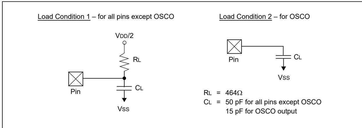
**TABLE 24-26: CAPACITIVE LOADING REQUIREMENTS ON OUTPUT PINS**
