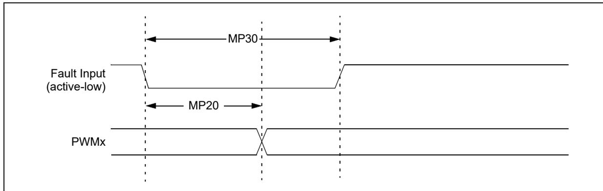
**FIGURE 24-6: HIGH-SPEED PWMx MODULE TIMING CHARACTERISTICS**
