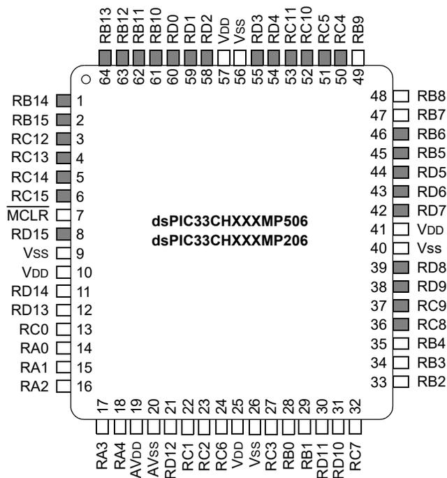
**Note 1:** Shaded pins are up to 5.5 VDC tolerant (refer to [Table 3-29](#)). For the list of analog ports, refer to [Table 3-28](#) and [Table 4-25](#).
