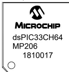
64-Lead QFN (9x9x0.9 mm)
