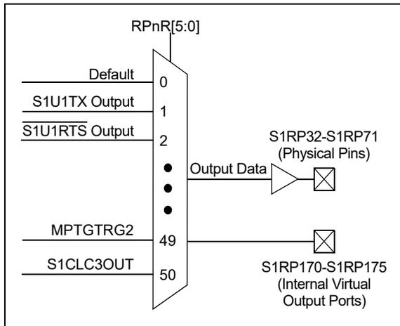
**Note 1:** There are six virtual output ports which are not connected to any I/O ports (S1RP170-S1RP175). These virtual ports can be accessed by RPOR20, RPOR21 and RPOR22.
