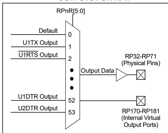
**Note 1:** There are six virtual output ports which are not connected to any I/O ports (RP176-RP181). These virtual ports can be accessed by RPOR20, RPOR21 and RPOR22.
