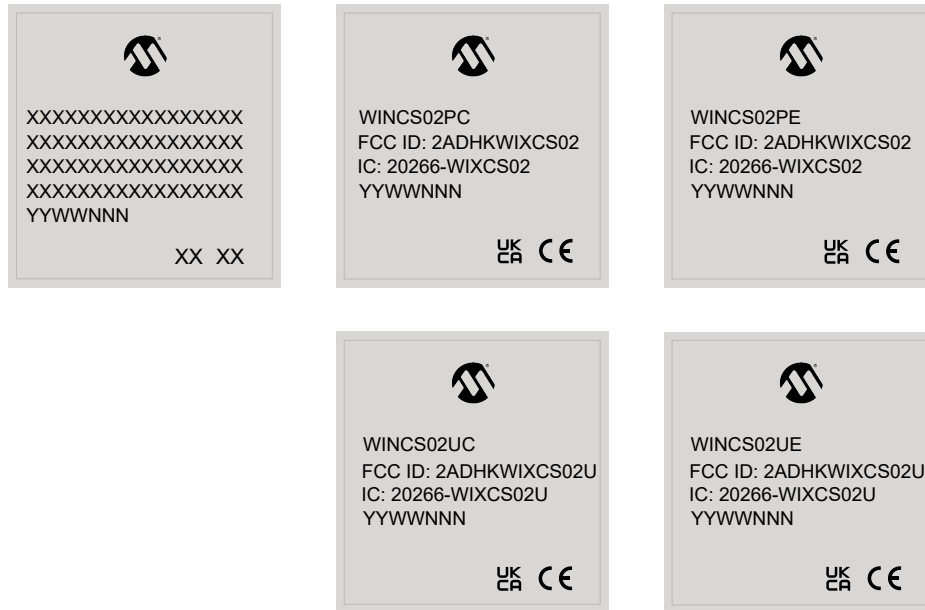
Figure 4-2. WINCS02 Module Packaging Marking
