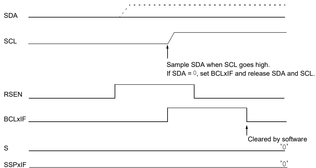
Figure 30-37. Bus Collision During a Repeated Start Condition (Case 1)
