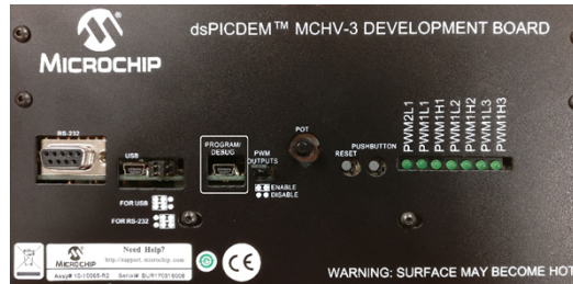
Figure 2-1. dsPICDEM MCHV-3 Development Board I/O Interface
