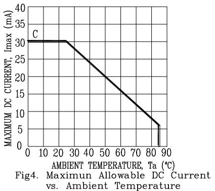
Fig4. Maximum Allowable DC Current
