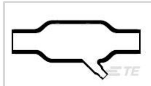
Molded Part Shape: **Y Shape**Number of Branches & Legs: **3**Material Code: **25**Material Systems Code: **25**Adhesive Requirement: **Adhesive Precoat**
