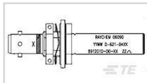
Contact Type: **Pin**Impedance: **3000 Ω**Data Bus Connector Style: **Bayonet**Data Bus Connector Type: **Jack**Polarization Code: **A**
