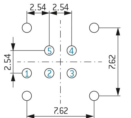
Contact borehole 0.8 mm Fastening borehole 0.8 mm
