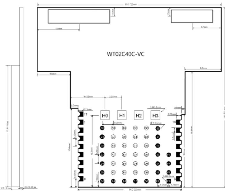
WT02E40C mechanical drawings, top view.
