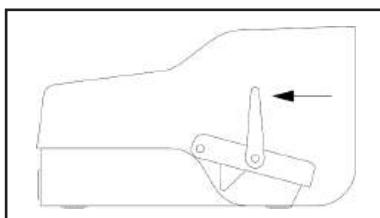
**Step 1:** To depress the pedal, the Anti-Trip lever must be pushed forward. Otherwise, a spring loaded mechanism holds the lever in position.
