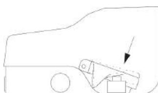
**Step 2:** To start the machine, the pedal must be depressed until the “pressure point”, where resistance is noticeable.
