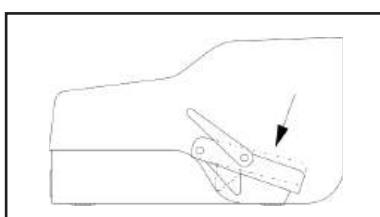
**Step 2:** After the lever is pushed forward, the pedal can be easily depressed.
