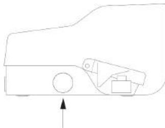
**Step 4:** The push button on the side of the foot switch must be pushed by hand to enable the foot switch to start the machine function again.
