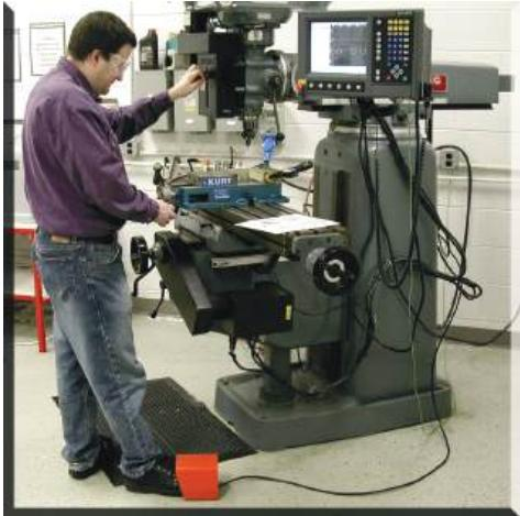
Altech's new low cost foot switch is ideal for any light to medium duty application. The PCFS-3M has an electrical rating of 10A (1/2HP)/125V AC, it can serve as a foot operated on/off switch for a wide range of motor driven and electrical devices.
