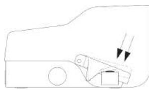
**Step 3:** In an emergency, if the pedal is depressed beyond the pressure point, the machine will stop. Beyond the pressure point, the contacts are locked in the “OFF” - Position. The machine cannot operate at this time.
