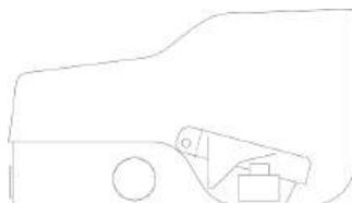
**Step 1:** The pedal is not depressed. The contacts are open. The machine is turned off.
