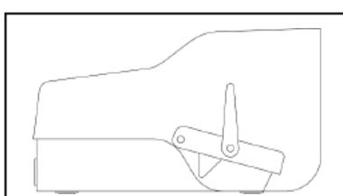
**Step 3:** Immediately after releasing the pedal, the spring loaded mechanism brings the lever back to its starting position.
