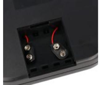
Four AA battery clips are supplied with S battery door sizes and eight clips are
