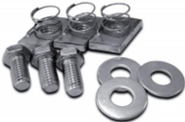
The 1463S is a hardware kit used to mount rack rails and other vertical rack accessories to Hammond cabinets. The 3/8 x 16 spring-loaded nuts install in seconds and simply push-in and rotate to secure in place into the rack cabinet ganging kit "C" channels.
