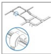
Movable exit maintains a proper bend radius for fiber optic cables that are routed over the side of your fiber management system.
