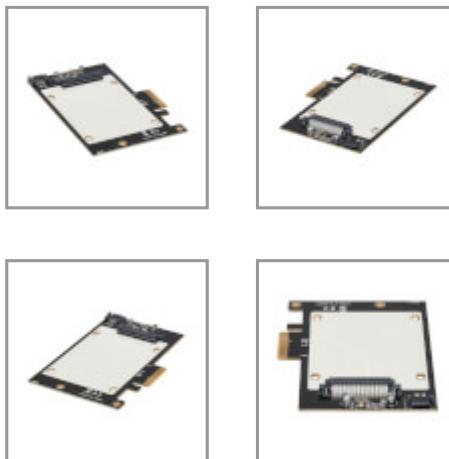
Mounts a NVMe U.2 SSD inside your PC or server to increase data transfer speed and internal storage.
