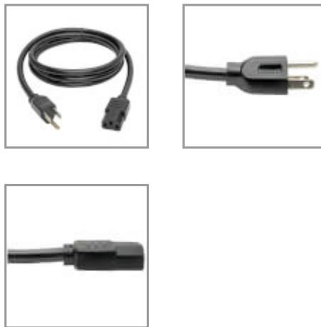
Computer power cord connects a server, computer, monitor, printer or other device with a C14 inlet to an AC outlet on a PDU.
